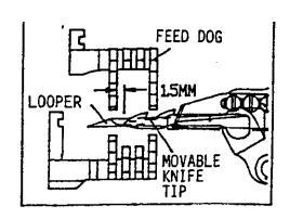
WHEN ADJUSTING, LOOSENING THE SET SCREW (A) AND TURNING THE ECCENTRIC STUD AND SETTING THE POSITION OF THE TIP OF MOVABLE KNIFE (THE SET MARK OF THE ECCENTRIC STUD MUST FACING TOWARD THE RIGHT SIDE).
